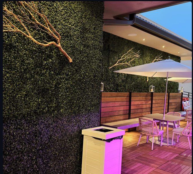
Deck seating: soffit downlight, wall-wash on the hedge, accent under the seating.
